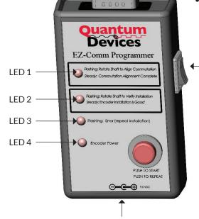
Plug power supply cube into 110 VAC supply. Connect +9v DC power plug into socket.
