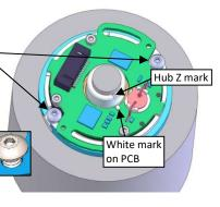
Place cover on encoder. Observe the cover dowel pins positioned into mating PCB holes.
