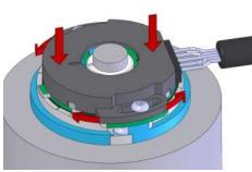
c.) Rotate encoder to align commutation channels to motor windings. Tighten cover screws to 37-43 oz·in.
