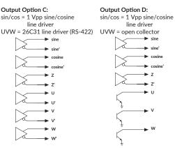
• 26C31 line driver is TTL compatible (can be wired single-ended)
