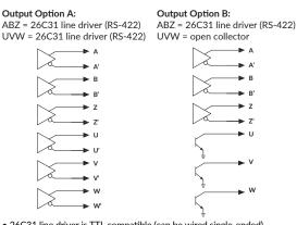
\* U', V' and W' are "no connect" for Output option B (open collector UVW)
