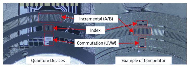
The effective sensing area of the A/B incremental channels on the Quantum Devices QML35 encoder (above, left) is 54% larger than Competitor's Encoder B (above, right).
