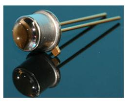
The LED in the Quantum Devices QM35/QML35 design is mounted to the PCB. A traditional transmissive optical encoder design is used, whereby the light source is located directly above the sensor, and the code disc sits in between the two. The following shows an LED package as mounted in a QM35 PCB:
