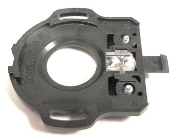
Overall, these design differences introduce several potential failure modes in Competitor's Encoder B design which are not present in the Quantum Devices QM35/QML35 LED. This includes: debris on the LED die obstructing or significantly blocking the light source, variations in location of the LED with respect to lens (in all three directions), susceptibility of color changes in the plastic lens and deterioration of LED die and/or connections due to environmental concerns.
