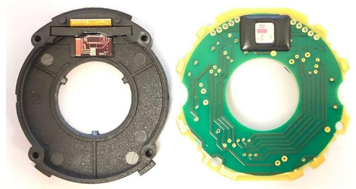
The sensor on the QM35 is Quantum Devices' patented interlaced photodiode specifically designed to translate light intensity to electrical current. The sensor is adhered to the polymer sensor base, and the electrical contacts are made with an elastomer multi-wire connector. All the connections are gold, and redundant wires connect to each of the sensor signals with the connector compressed between large pads on the sensor and PCB.
